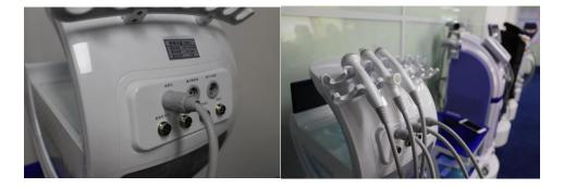
Installation of 2) high-frequency spatula, ultrasonic waveguide head, gold radio head, camera First find the corresponding hand gear connection line and the corresponding plug, the plug groove position is aligned to the left clasp position of the connecting hole, push hard inward, and then tighten the nut counterclockwise after fastening.
