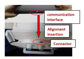
3. Insert the power connector into the connection port
